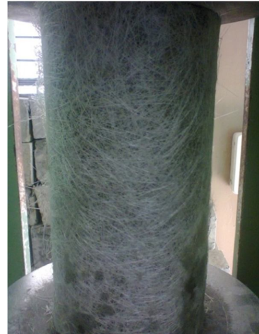
Figure 1: FRP Confined Specimens
